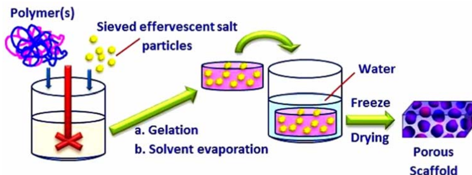
Figure 11. Schematic illustration of gas foaming-leaching technique for fabrication of porous hydrogel scaffolds for tissue engineering applications.
