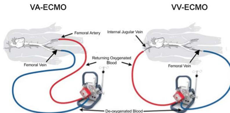
**Figure 9. Veno-Arterial and Veno-Venous: Extracorporeal membrane oxygenation circuit.**
