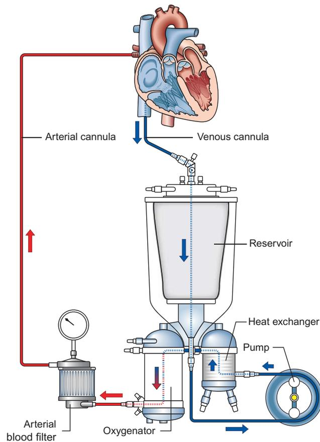
**Figure 2.** Overview of cardiopulmonary bypass circuit and its various components.
